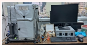
High Pressure Visual cell with interfacial tension, contact angle and drop volume measurement system
